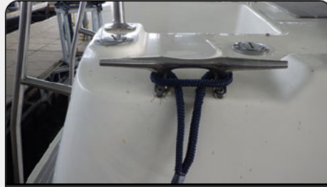
Photo 13: Cleat showing signs of cracking.
