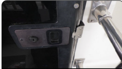
Photo 43: lock broken on companion way entrance
