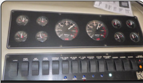
Photo 20: Instrument display during trial run. Note rev difference between engines.
