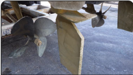
Photo 16: General view of props and rudders showing good condition of props and rudders. Note: smallest nut should be closest to prop as per ABYC.
